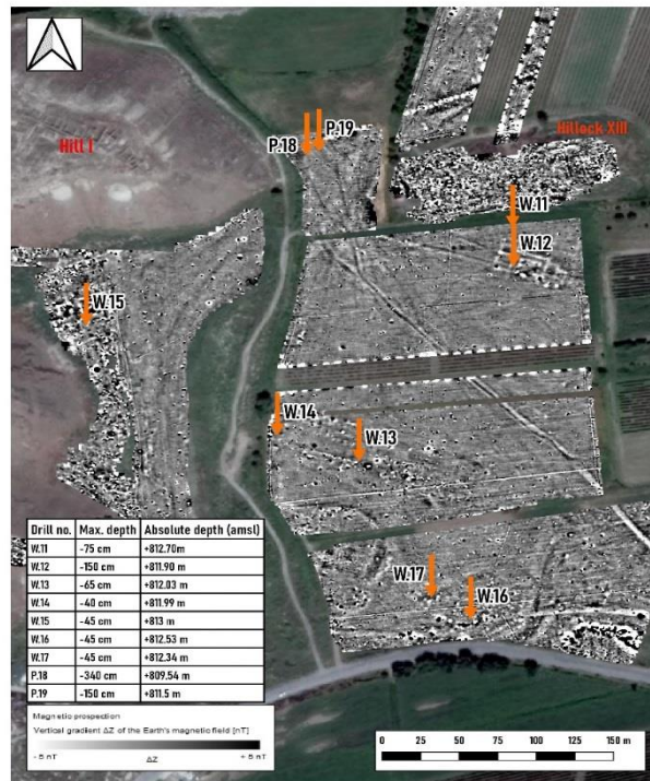
Figure 10: Map showing the locations and depths of all the single drills, plotted on the 5nT magnetic map (Eastern Atlas; N. Noorda)
